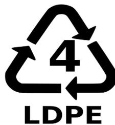
**Gambar 2.7** Kode Plastik Jenis Low Density Polyethylene (LDPE)
