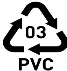
**Gambar 2.6** Kode Plastik Jenis Polyvinyl Chloride (PVC)
