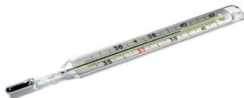
Gambar 2. 2 Termometer Raksa (Suparno, 2009)
