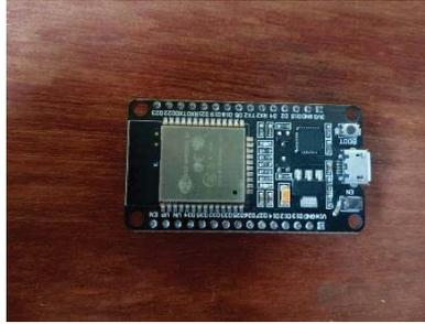
Gambar 2.4 NodeMCU ESP32
