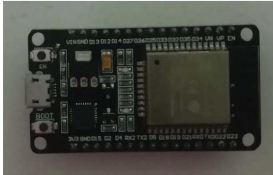
**Gambar 2.3** NodeMCU ESP32
