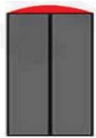
**Gambar 2.10** Sambungan tekuk (*edge joint*)
