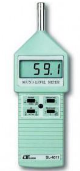
Gambar 2.5. Sound Level Meter
