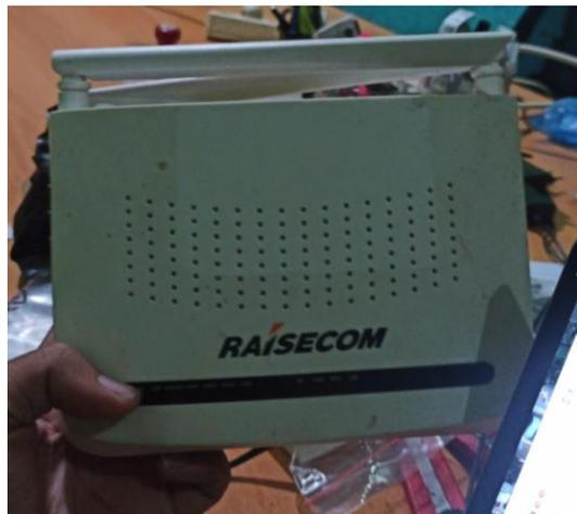
**Gambar 2.34** *Optical Network Termination (ONT)*
