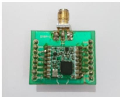
**Gambar 2.4** Modul *Transceiver* SX1276
