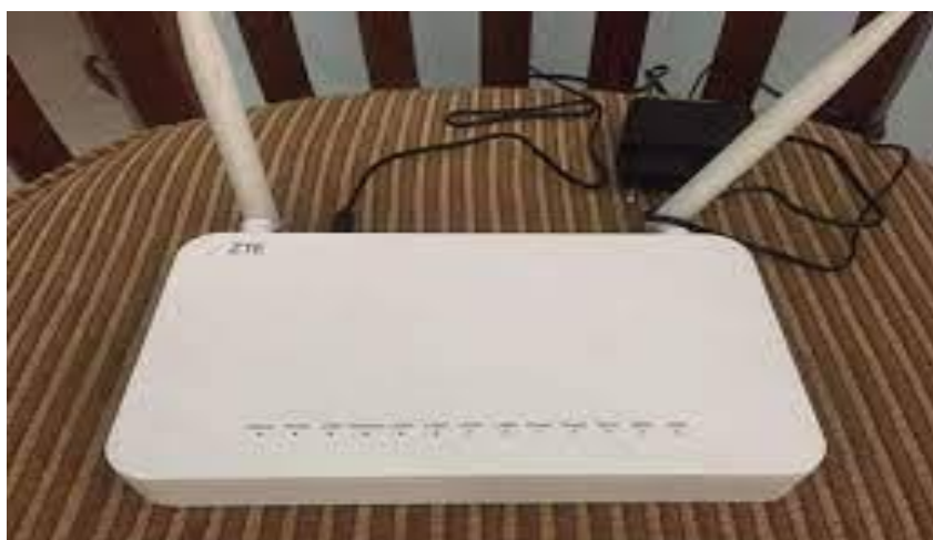
Gambar 2.10 ONT ( Optical Network Termination )
