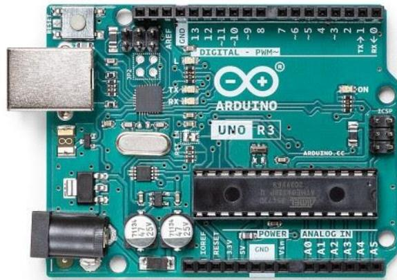
**Gambar 2.1** Arduino Uno board
